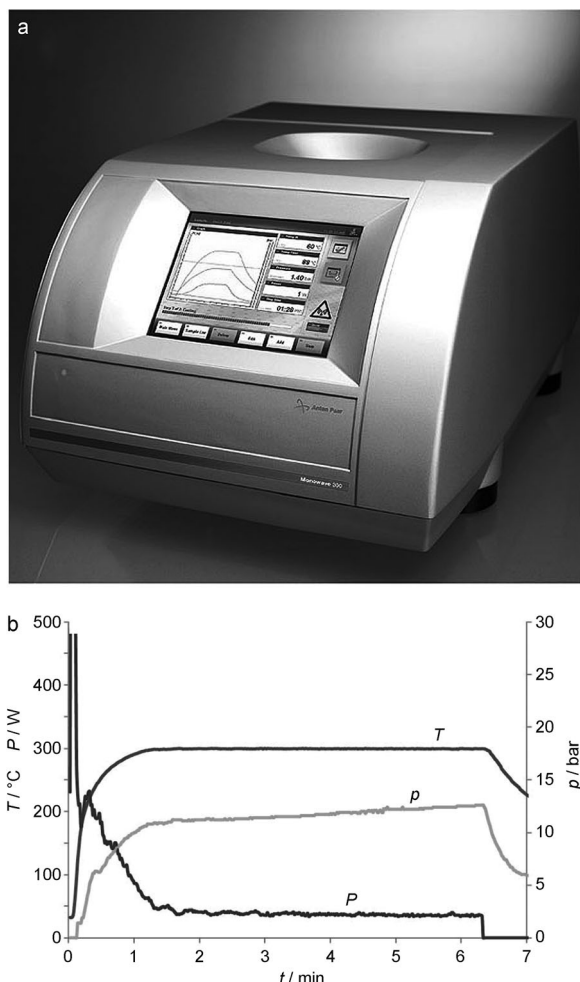
Figure 1. a) Photograph of a single-mode microwave reactor (Monowave 300, Anton Paar GmbH, Austria) capable to operate at up to 850 W magnetron power and equipped with a dual internal/external temperature monitoring system. b) Temperature ( T ), pressure ( p ), and power ( P ) profiles recorded for a 3 mL sample of ethylene glycol MW-heated under sealed-vessel conditions to 300 °C in the Monowave300 reactor. For the sake of clarity only the internal fiber-optic probe temperature profile is shown and the y-axis has been cut at 500 W.
